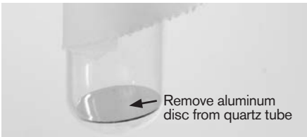
Fig. 6 (Older Ultra UV, discard aluminum disc)
